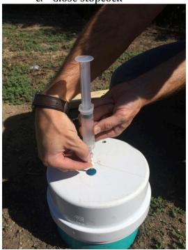
d. Remove needle from septum by holding NEEDLE (not syringe or stopcock) with two fingers and placing a finger or two on the septum to prevent it from pulling out of chamber top.
