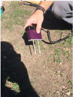
Make sure rods are straight and not bent. Replace if bent.
