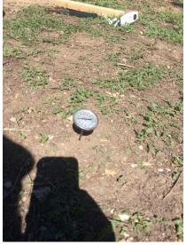
Record air temperature by using thermometer in the shade at chamber height level. Once per sampling in middle of measurement period (for that group of 6) is sufficient. Record in notebook.
