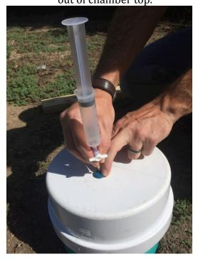
e. With stopcock CLOSED, press on plunger to 17 mL, creating positive pressure in
