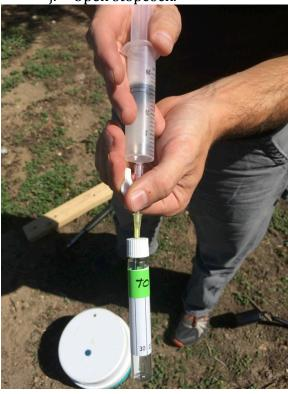
k. Push sample into Exetainer. You should feel or see the negative pressure in evacuated Exetainer pull the syringe plunger. If you do not see or feel pull, you have one of two problems: No vacuum in your Exetainer or a sticky syringe. Replace the syringes regularly (after 1-2 sampling dates) so they are well lubricated and not sticky. If the plunger does not move, immediately close the stopcock and use a new exetainer (always bring spare Exetainers and label appropriately).
