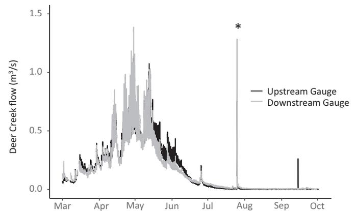
FIGURE 3. Hydrographs for 2013. Between May 16 and June 15, inflow to the meadow (black) exceeded outflow (gray). After June 15, outflow exceeded inflow. A brief, intense flood on July 26 (\*) peaked at  $4.3 \text{ m}^3/\text{s}$  at the downstream gauge and  $2.8 \text{ m}^3/\text{s}$  at the upstream gauge. These peaks were removed in further analyses.
