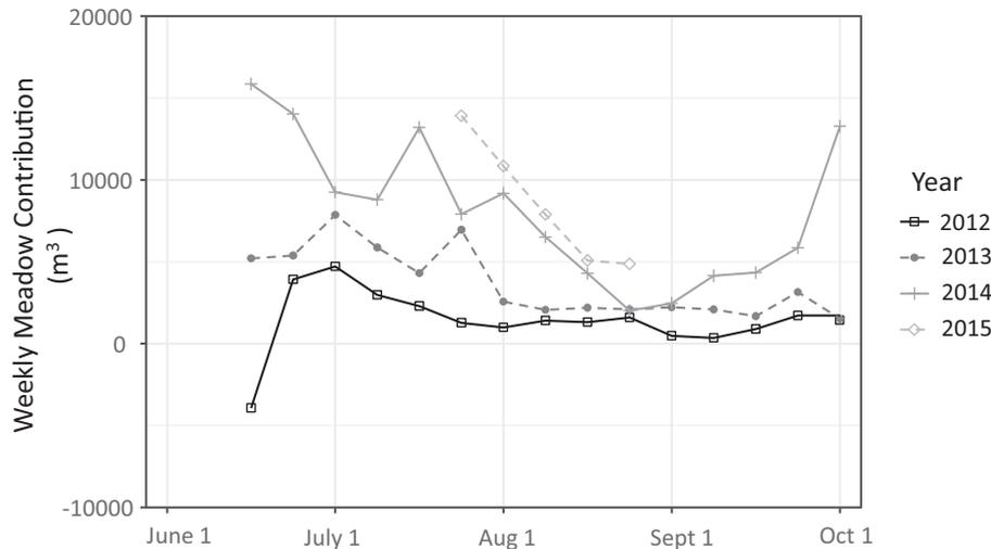
FIGURE 4. The weekly meadow contribution ( $\text{m}^3$ ) is the difference between cumulative outflow and cumulative inflow for one week. Values after restoration (2013–2015) exceeded values before restoration for 14 out of 15 weeks during the low-flow period.
