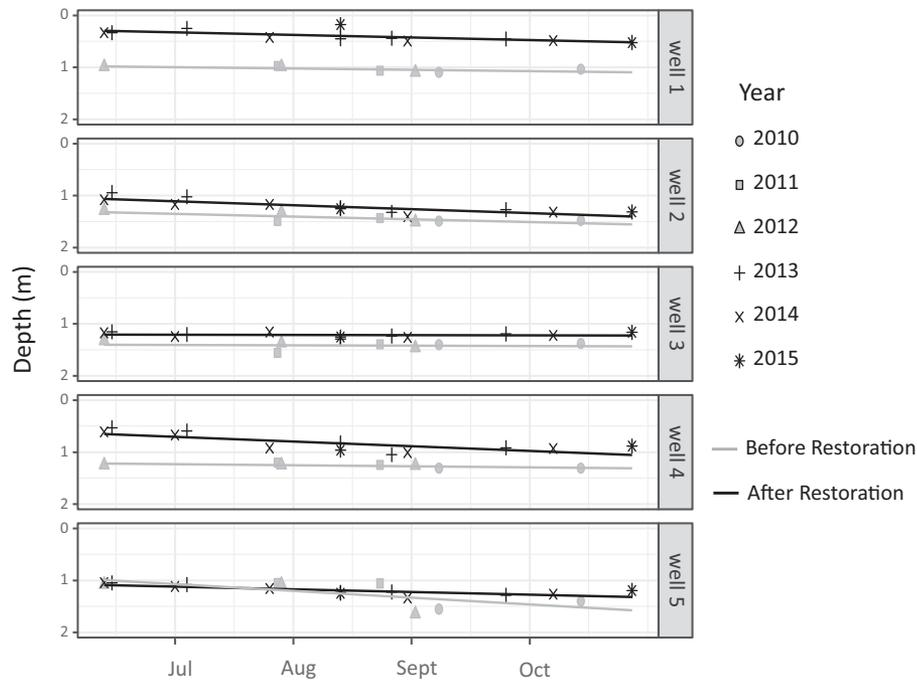
FIGURE 5. Groundwater elevations after restoration (black) were higher than before restoration (gray) for Wells 1–4 (ANCOVA,  $F > 32$ ,  $p < 0.001$ ). Regression lines combine data for the years before restoration (2010–2012, filled symbols, gray lines) and after restoration (2013–2015, black lines). ANCOVA, analysis of covariance.
