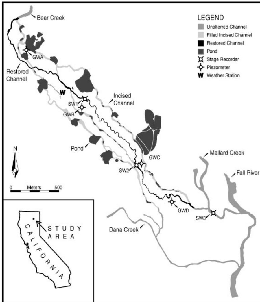
Figure 1. Bear Creek Meadow study area. Portions of the incised channels were filled with alluvium excavated from ponds throughout the meadow. A 3.6 km single thread restored channel reach was created from remnant channel segments and excavated where necessary. Flow direction is from upper left to lower right. Surface and groundwater comparison locations are also shown
