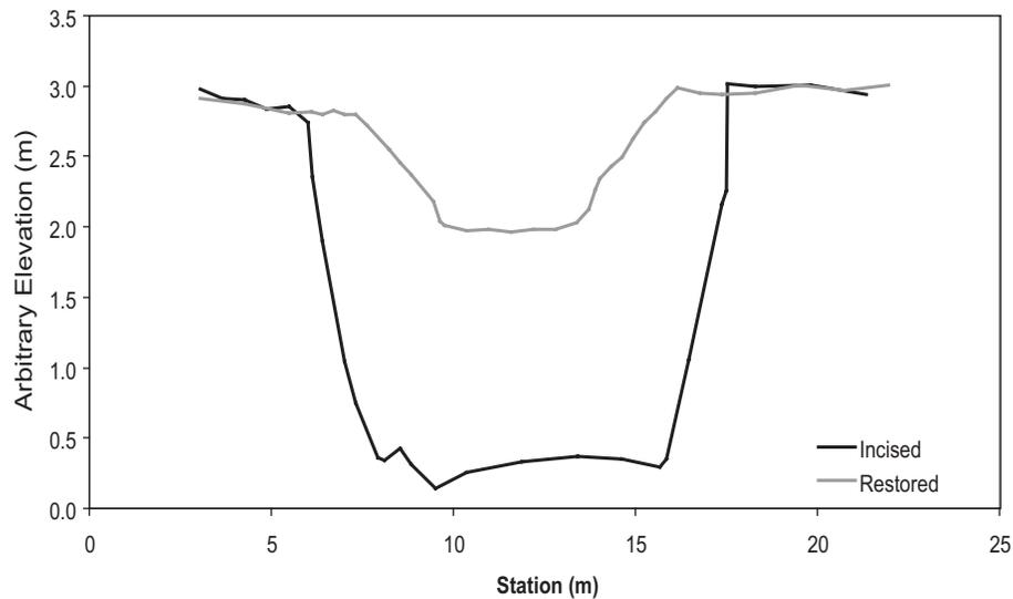
Figure 4. Representative restored and incised cross sections of the Bear Creek channel
