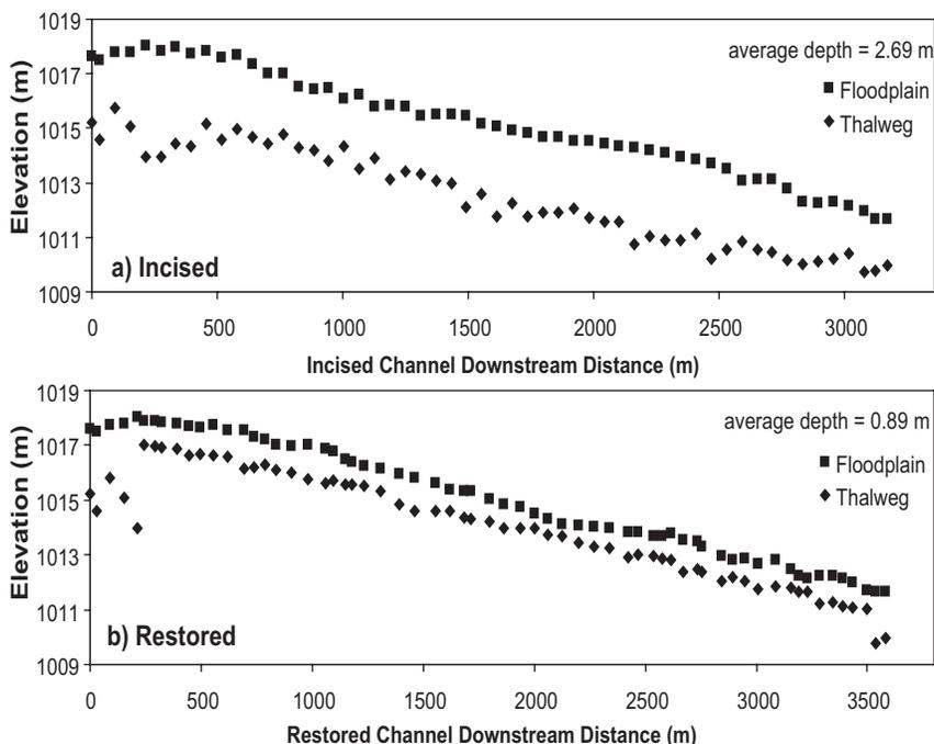
Figure 3. Long profiles of riffle crest thalweg and adjacent floodplain elevations for (a) incised and (b) restored channel geometries. The restored reach begins at restored channel station 800 m and ends at restored channel station 3535 m corresponding to incised channel station 800 and 3124 m, respectively. The first five and last two points in each of the surveys represent identical locations
